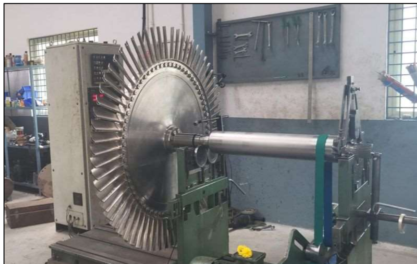
Figure 5-4 – The Kavaratti OTEC project has achieved a significant milestone with the successful dynamic balancing of its 65 kW Open-Cycle turbine's rotating components. Ref. National Institute of Ocean Technology (NIOT), Chennai, India
